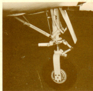
The rugged nose landing gear incorporates a gear door which functions as a cowl flap when the gear is retracted.
