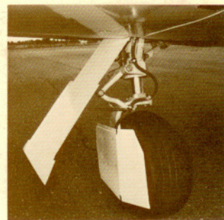
The main landing gear is completely enclosed in the retracted position to maintain the clean drag-free lines of the Eagle I.
