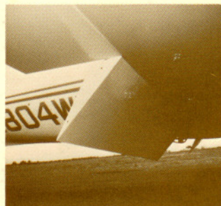
The rugged nose landing gear incorporates a gear door which functions as a cowl flap when the gear is retracted.
